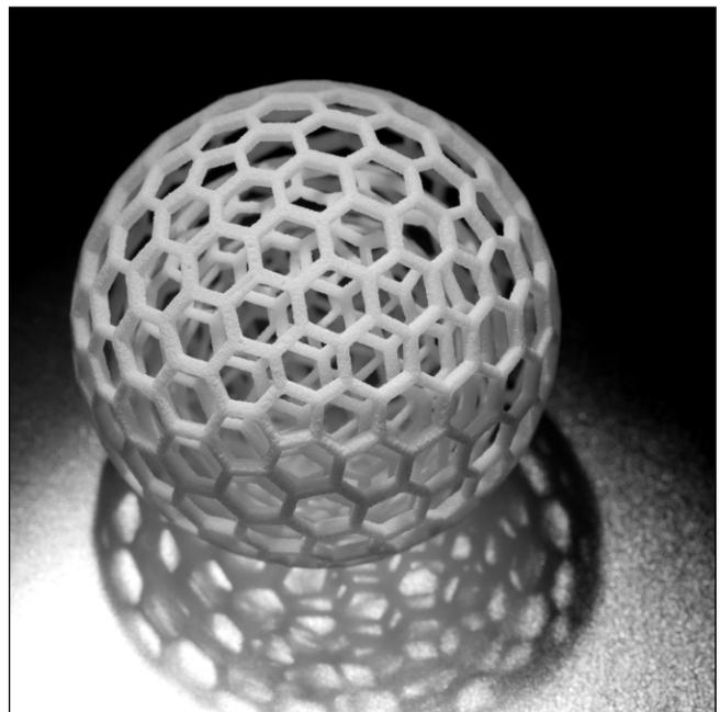
process that starts with nothing and builds the product by "printing" or depositing layers of material to the specifications shown on the digital design. Materials range from thermoplastics and polymers to ceramics,
